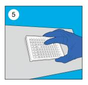
Tap the wells (face down) on a layer of absorbent paper to remove residual wash buffer.
