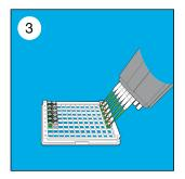
**A.** Use multichannel pipettor to mix by pipetting up and down, then transfer the standards and samples to the appropriate antibody coated wells.
