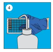
Decant the contents from the microwells into a discard basin. Wash the wells by filling with wash buffer, then decant the buffer into the discard basin. Repeat for 5 washes.
